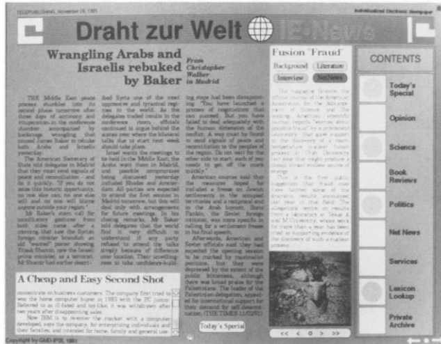
FIGURE 1. Interface for an “individualized” electronic newspaper designed by the IPSI Institute, Darmstadt. Clicking the buttons on the right brings up screen displays of different sections of the paper, or services like dictionaries and the user’s private archive. Clicking buttons marked “background,” “interview,” and so on brings up new windows containing related stories or information. The picture is actually a single frame of a video. The newspaper is available in several display formats.
